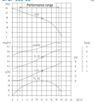
Total performance characteristic of the pump is given in the informative diagram. Informative total characteristic Q-H corresponds to pumping clean water of density  $p = 1,000 \text{ kg.m}^{-3}$ . With increasing density of a pumped liquid the power input P, could increase too.
